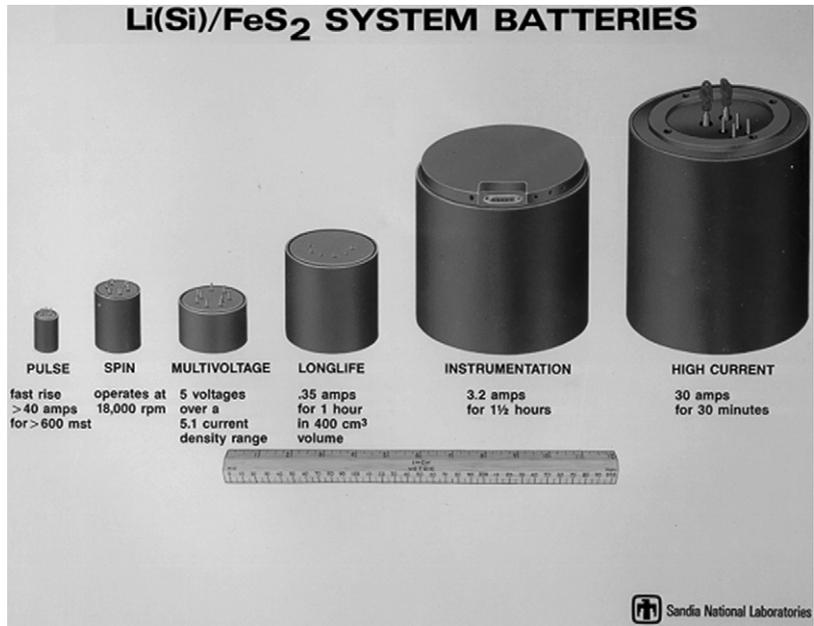
Fig. 1. Photograph of the wide variety in sizes of Li–Si/FeS<sub>2</sub> thermal batteries developed at Sandia (a 12-in. ruler is shown for size comparison).
